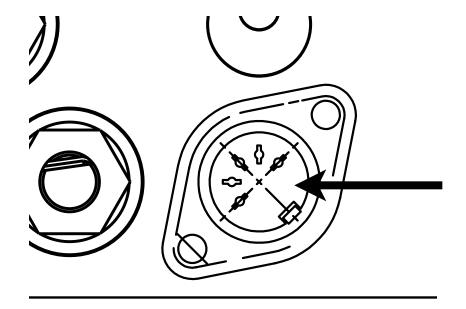
Step Three: Plug your instrument signal into the Input Jack of the Programmable Bypass Looper. You can directly connect your instrument (Guitar, Bass, Etc.) to the Programmable Bypass Looper, or you can connect from another pedal or device used inline. The Programmable Bypass Looper does not need to be first in the signal chain.
