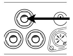
• Step Five: Connect the proper power to each pedal being used, including the Programmable Bypass Looper. The Programmable Bypass Looper requires a power supply of 9V DC, and uses a tip negative polarity. It is recommended to use a power supply that supplies 400mA of current or more.
