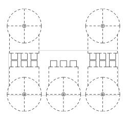
Horizontal Knob Separation: 0.8" (bottom) Horizontal Knob Separation: 1.6" (top) Vertical Knob Separation: 1.4"
